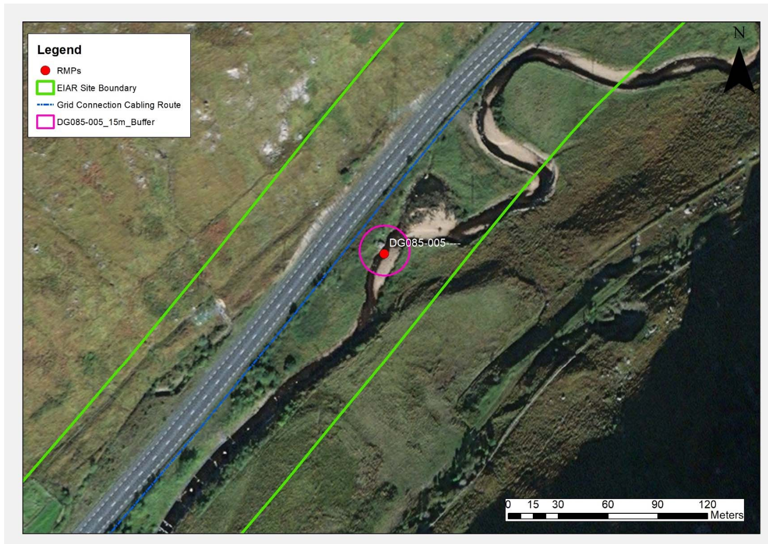
Figure 13.9: DG085-005 megalithic structure 'site' showing 15m protective area. Fencing along the roadside during construction outside this zone.
